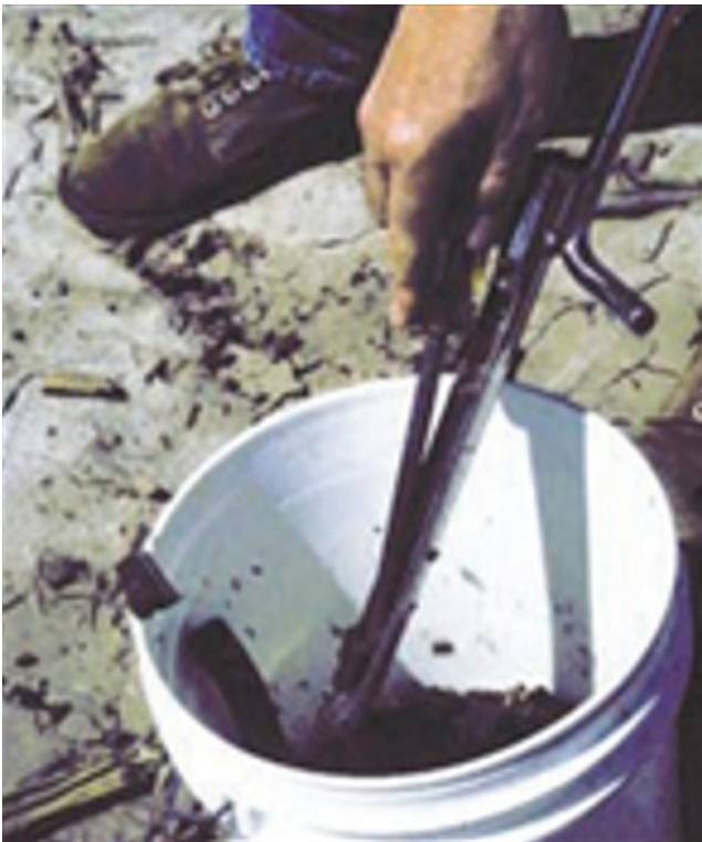
Fig. 15.10. Tools recommended for soil sampling for soybean cyst nematode: soil-sampling probe, screwdriver to remove soil from the probe, and bucket to bulk individual cores. (image: Illinois Agronomy Handbook, 2009 Edition)
