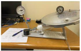
Testing takes about 15 minutes and ensures your dial gauge reads correctly. Inaccurate gauges can result in under-processed foods, which can pose serious health risks like botulism.
