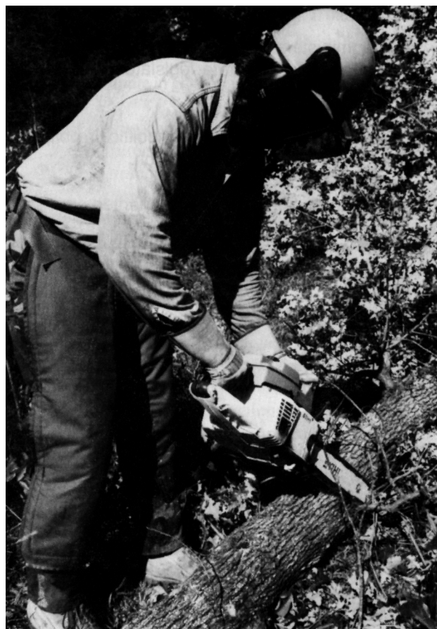
Figure 4. In limbing a fallen tree, keep the saw chain on the opposite side of the log being worked on when possible. This will help prevent accidental contact with the saw chain.
