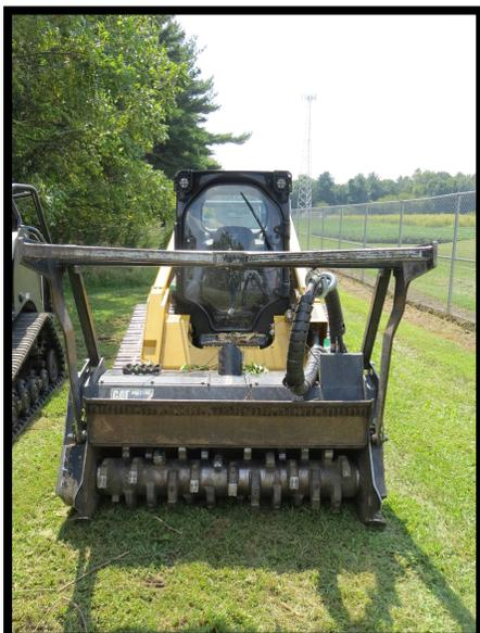
Caterpillar skid-steer with a Fecon™ mounted mulching head used to clear understory bush honeysuckle from UI experimental forest.
