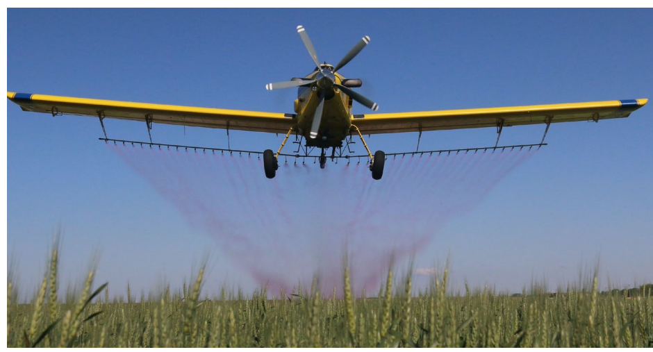
Air Tractor AT-802A pattern testing, Matt Gill, University of Illinois.
