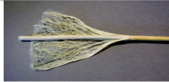
Hemp Stalk: Bast and Core Photo Credit: Hemp Gazette
