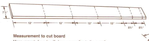
Measurements for cuts will change according to the overall dimensions of the box you want to make. This illustration shows how to make cuts for a box that is 12" long x 7.5" high x 6" deep.
