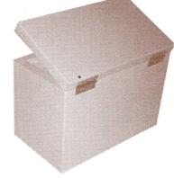
\* Please note: Finished lumber, although sized as one inch in its depth (also referred to as a "one by") is actually 3/4", not a full one inch. The measurements given here are using a 3/4" depth size.
